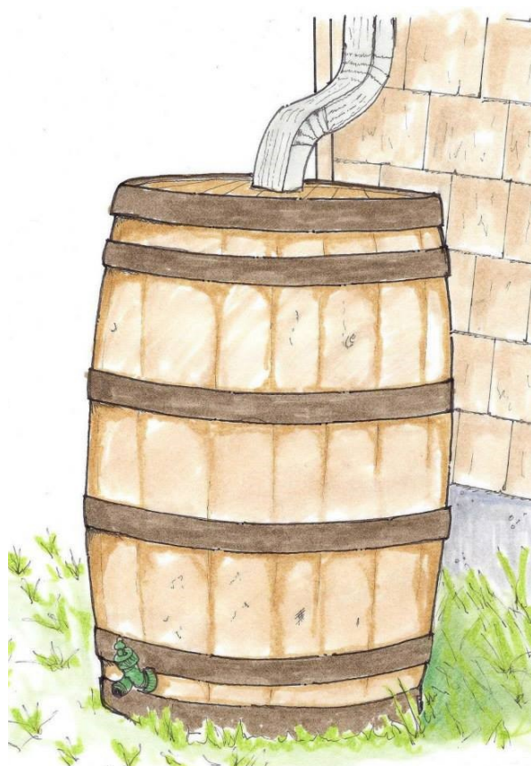
Sketch of a rain barrel, an example of rainwater harvesting. Photo from Soak Up The Rain New Hampshire
